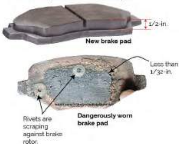
New brake pad versus worn brake pad
