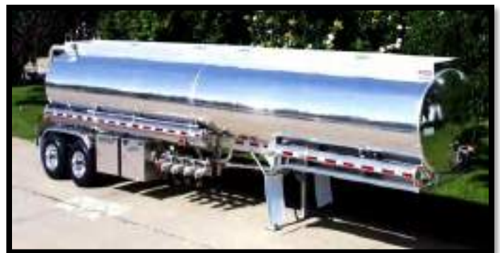
Fuel Trailer with bulkheads can carry different grades of fuel
