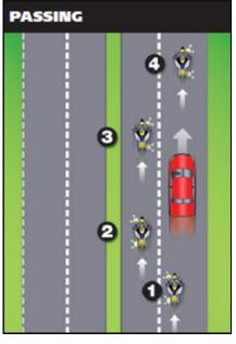
vehicle that is traveling below the posted speed limit on a 2-lane highway. The posted speed limit must be 55 mile per hour or greater. Not allowed in work zones. It is never a good idea to pass on a bridge, blind hill, or any other time your sight distance and escape route is compromised.
